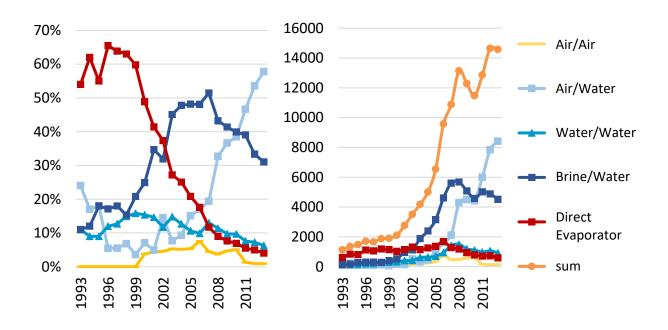
Figure 36: Sold heat pumps per year divided in the kind of source/sink systems in relative (left) and absolute numbers (right) (Rieberer, 2017)
