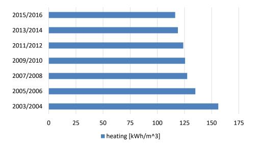
Figure 16: Final energy demand for heating in buildings per m3; data according to Statistik Austria (2017)
