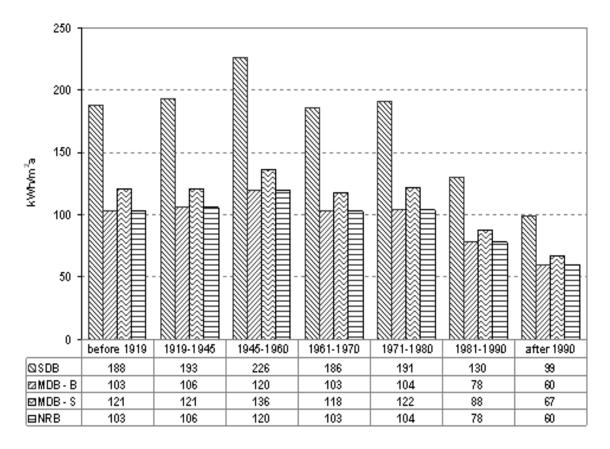
Figure 20: Specific annual energy use for heating in kWh/(m2\*a) of single (SDB) and multi-dwellings (MDB; -B = Large, -S = Small) buildings, as well as non-residential buildings (NRB) by the construction period (Moisi et al., 2015)
