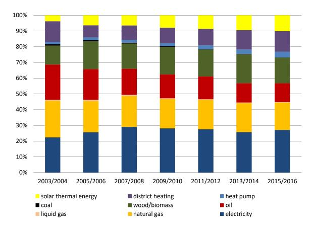
Figure 29: Relative usage of all energy sources for DHW heating; data according to Statistik Austria (2017)
