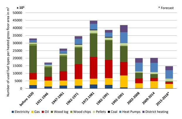
Moreover, Figure 25 shows the same data as used in Figure 24 in absolute numbers, to give an overview of how many square metres are heated with which kind of energy source.
