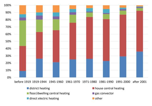
Figure 21: Heating systems in the building stock according to the construction period; data according to Statistik Austria (2016)
