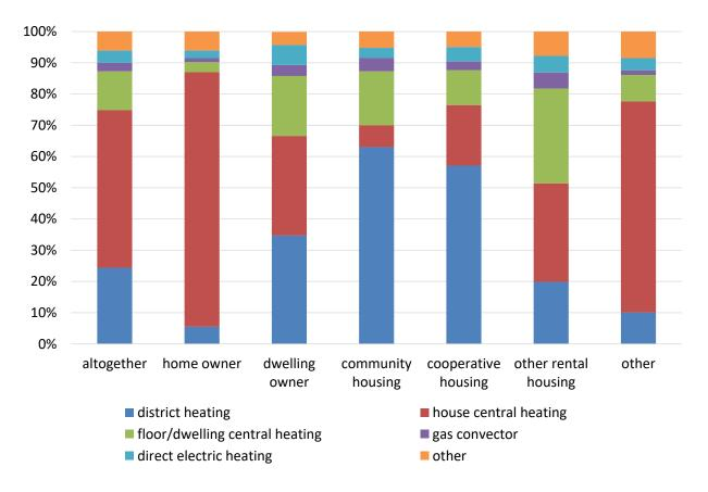
Figure 22: Heating systems in the building stock according to the type of ownership; data according to Statistik Austria (2016)
