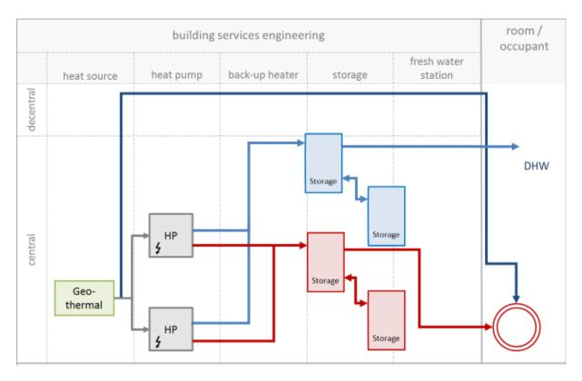
Figure 60: System layout of the system in Villach
