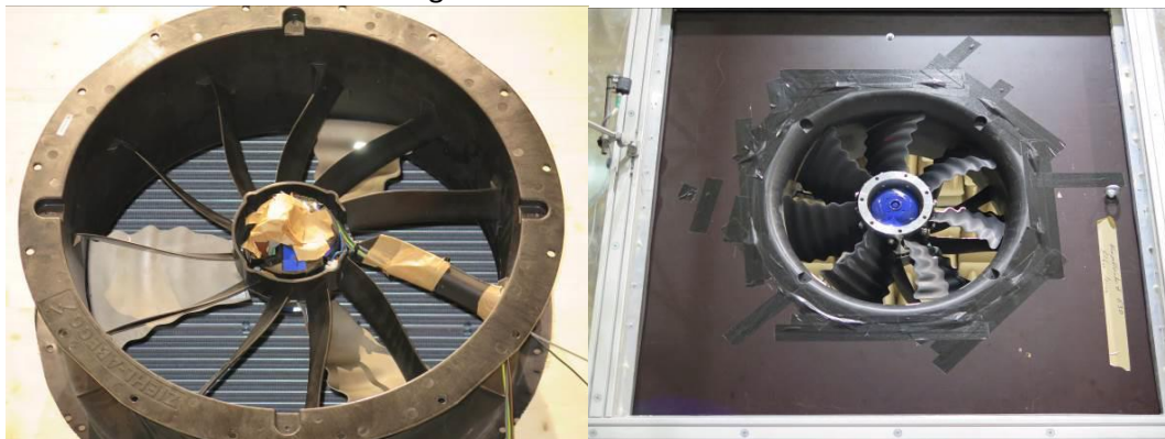
Figure 5.11: Fan prototypes for EC090 drive (left) and EC116 drive (right) with tonal noise reduction technique (from the FP7_GreenHP Project, Deliverable 7.1)
