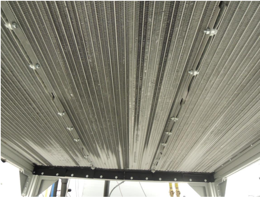
Figure 5.10: Icing of the GreenHP heat exchanger (enlarged view, with ice)
