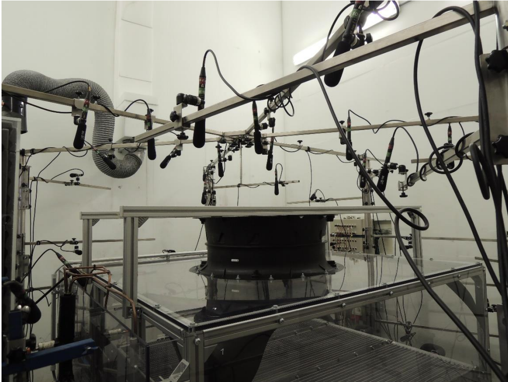
Figure 5.2: Acoustic Dome surrounding the GreenHP (view to the upper part)
