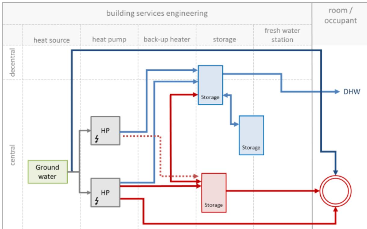
Figure 54: System layout of the system in Simmering
