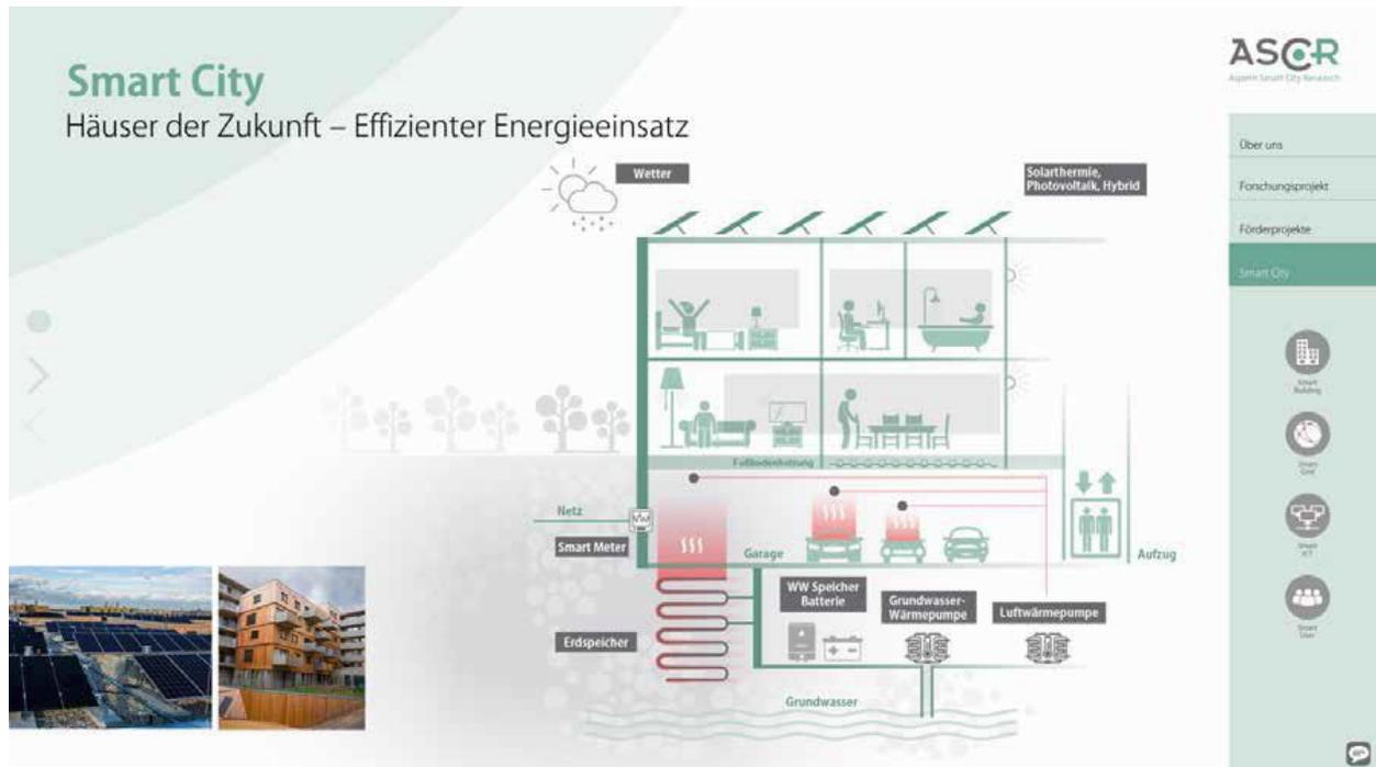
Figure 51: Schematic diagram of the heating system in the Smart City Aspern (Niederbrucker et al., 2016)
