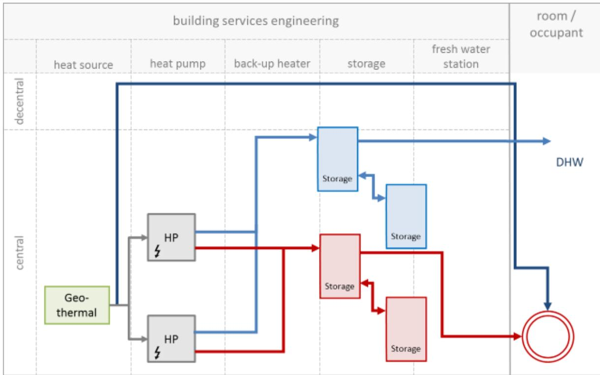
Figure 60: System layout of the system in Villach
