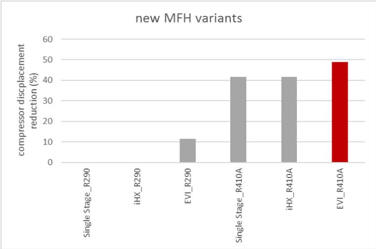
Figure 15: Compressor displacement reduction for new MFH variants
