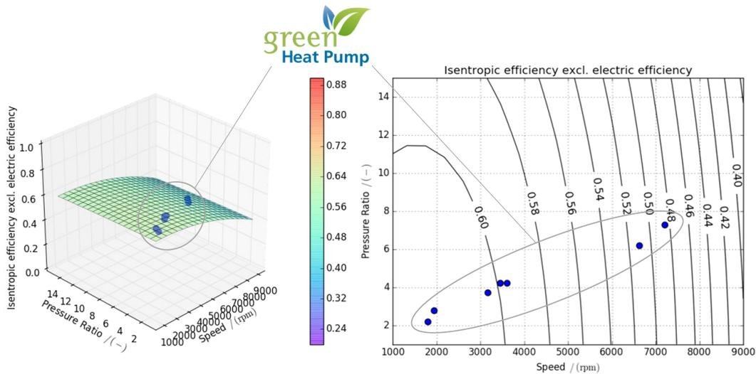
Figure 7: Calibrated isentropic efficiency with the GreenHP-measurement data (blue)
