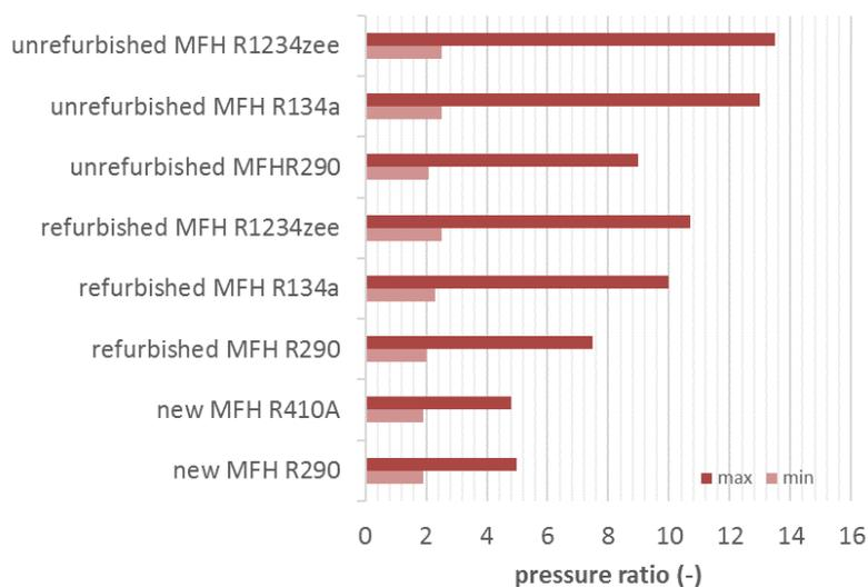
Figure 14: Pressure ratio depending on refrigerant and use case
