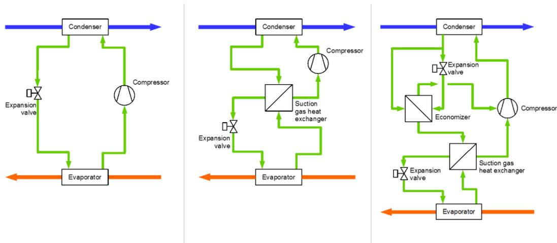
Figure 2: Refrigerant circuit configurations, from left to right: single stage, suction gas HEX, EVI
