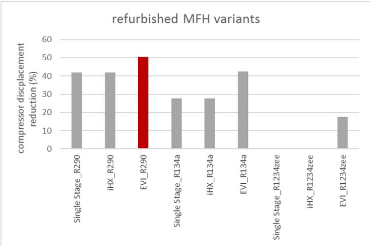
Figure 16: Compressor displacement reduction for refurbished MFH variants
