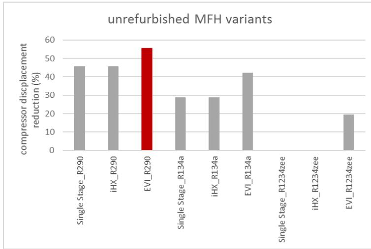
Figure 17: Compressor displacement reduction for unrefurbished MFH variants
