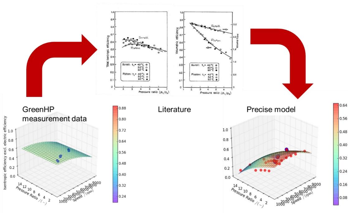
Figure 8: Generation of an improved compressor maps: GreenHP-measurement data combined with literature.
