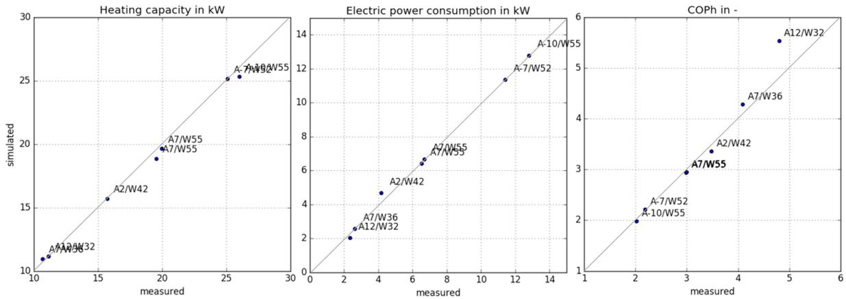
Figure 5: Validation of the numerical model with the GreenHP-measurement data
