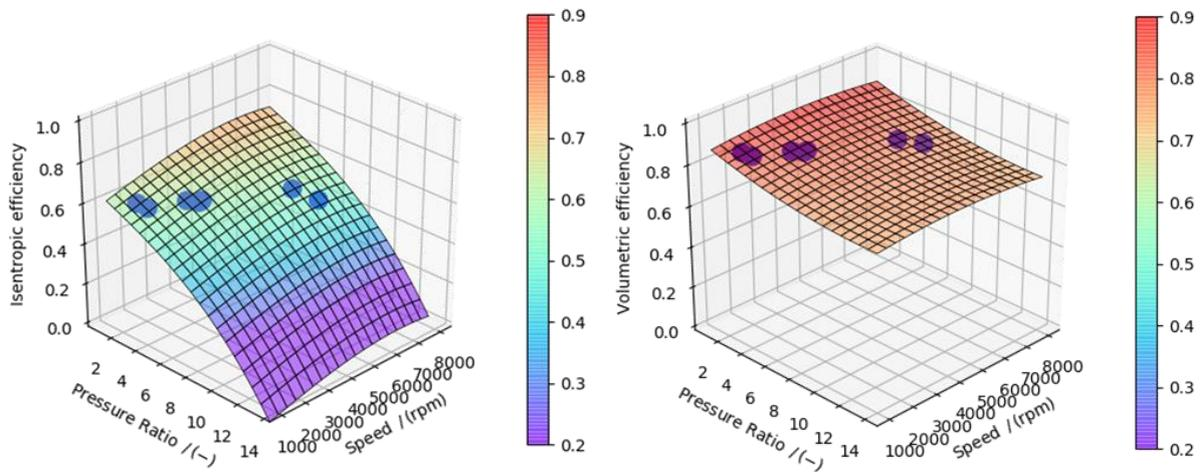
Figure 9: Improved compressor maps. Isentropic efficiency (left) and volumetric efficiency (right). The original GreenHP-measurement data are indicated as blue dots
