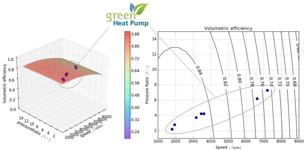
Figure 6: Calibrated volumetric efficiency with GreenHP-measurement data (blue)
