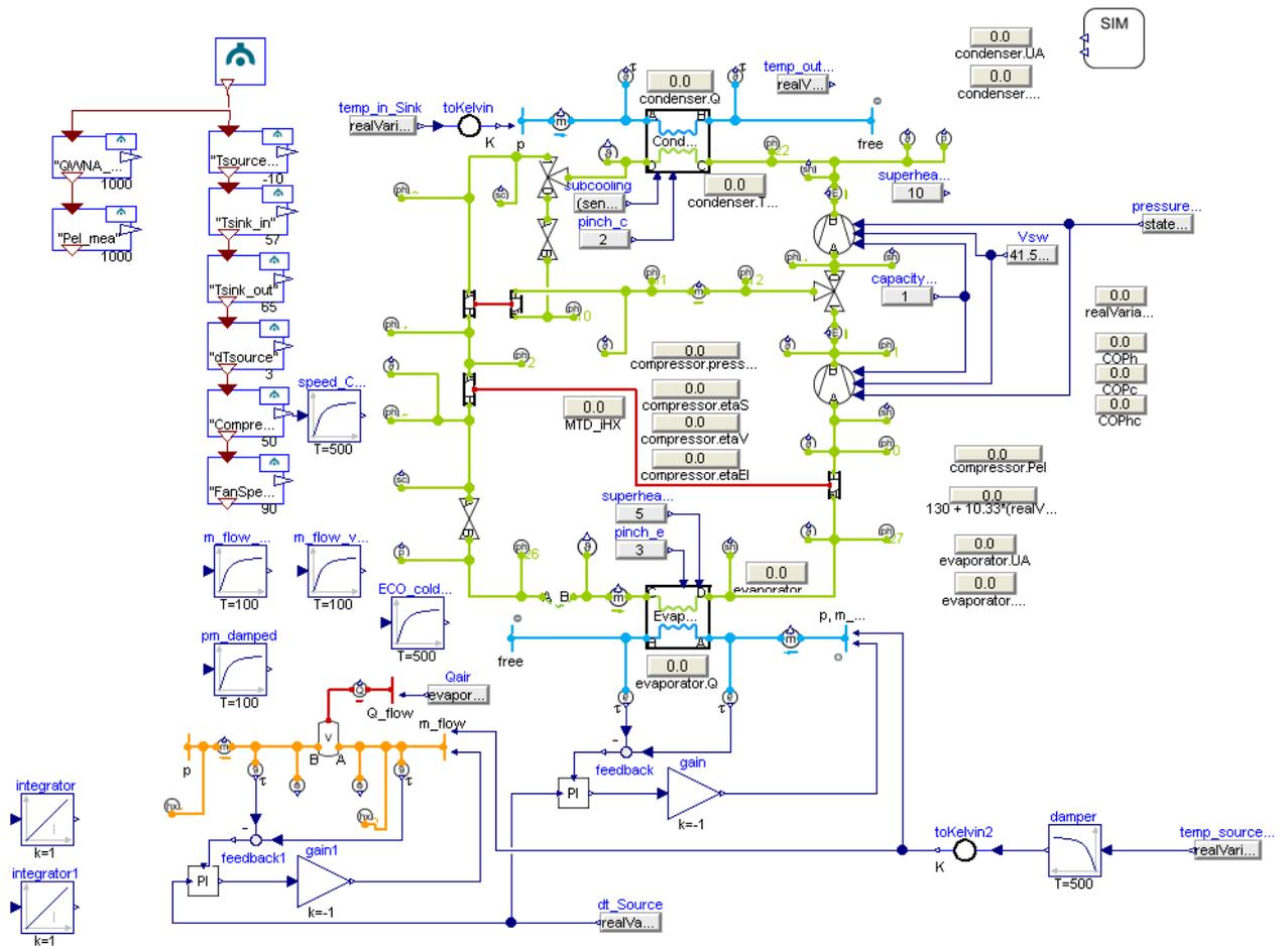
Figure 3: Numerical model in /Dymola/Modelica®
