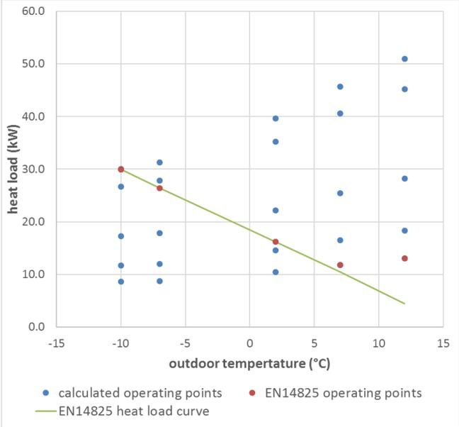
Figure 10: Operating map example for the variant refurbished MFH with EVI and R290
